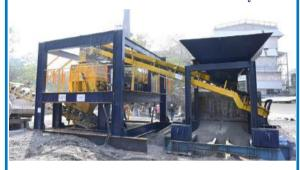
Bokaro: In a push to strengthen its raw-material processing capabilities, Bokaro Steel Plant (BSL) has commissioned a new 100-tonne-per-day lime crusher unit at its Raw Material Management (RMP) department. The facility, located at the lime discharge complex, was inaugurated by Executive Director (Works) Priya Ranjan, in the presence of Executive Director (Operations) Anoop Kumar Dutt and senior officers of BSL and FSNL.
